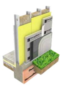
Steel studs, batt cavity insulation, glass-mat faced sheathing, EnergyShield Pro with taped joints, grade D building paper, expanded metal lath, cement plaster scratch and brown coats, stucco finish.
