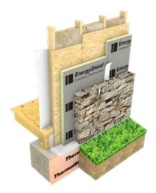
Wood studs, batt cavity insulation, wood sheathing, EnergyShield with taped joints, stone cladding.
