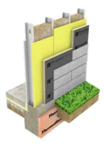
Steel studs, batt cavity insulation, glass-matt faced sheathing, EnergyShield CGF Pro with black facer side out and taped joints, metal panels installed with open joints.
