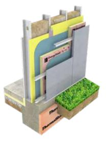
Steel studs, batt cavity insulation, glass-mat faced sheathing, liquid applied air & moisture barrier, EnergyShield Ply Pro, metal panels.
