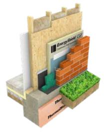
Wood studs, batt cavity insulation, wood sheathing, EnergyShield CGF, liquid applied air and moisture barrier, mortar net, brick.
